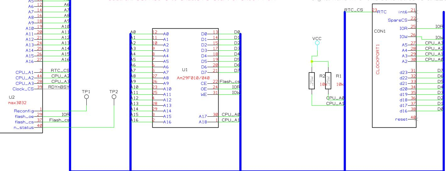
TP1 soldered to diodes right next to instant-on board TP2 soldered to nStatus signal on board (blue wire) RDYnBSY signal becomes DMA signal of expansion after config CPLD ignores RDYnBSY while doing config (writes are timed only) config data is taken from address 0x60000 of flash chip
